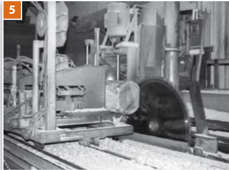
5 Logs were ripped into boards and slabs (5) which were dropped into a pit and chopped into bark mulch. Men stacked freshly-sawn boards (7) into "cubes" for drying. Cubes were made ready (8) to be picked up by forklifts and placed in the kilns.
