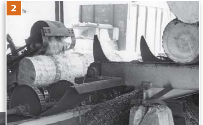
Logs started the production process in the newly-made log room (1) by being placed on the first live deck. The debarker stripped away the bark (2). Davis loaded debarked logs onto the second live deck (3) which sent them inside the factory.
