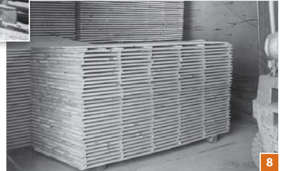
5 Logs were ripped into boards and slabs (5) which were dropped into a pit and chopped into bark mulch. Men stacked freshly-sawn boards (7) into "cubes" for drying. Cubes were made ready (8) to be picked up by forklifts and placed in the kilns.
