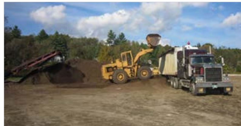
Below: The tub grinder in action (left). Steam rose from the mulch when it was disturbed. After the initial pass through the grinder, the building mulch was sent through a second time to generate a high-quality mulch. A loader (right) placed the refined mulch into a truck which transported it to locations throughout the valley.
