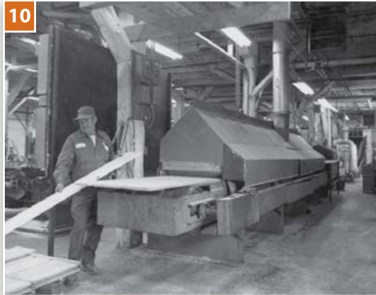
Dried boards from the kiln were fed onto a long machine via conveyor to undergo the critical phases of the not-so-secret process. First, the boards (10) were scratched by spinning wire brushes to create a weathered look. Next, the boards were stained (11). Haynes mixed his own stains in a large shower stall next to the machine (upper left of photo below). Then the boards were fed into a dryer (12).
