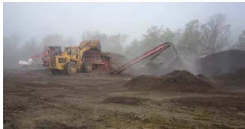
Below: The tub grinder in action (left). Steam rose from the mulch when it was disturbed. After the initial pass through the grinder, the building mulch was sent through a second time to generate a high-quality mulch. A loader (right) placed the refined mulch into a truck which transported it to locations throughout the valley.
